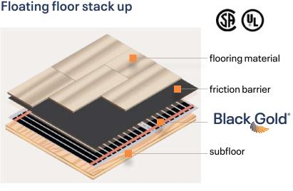
Black Gold film adds just 1/16" to the total floor stack up.\* \* Total stack-up varies with flooring material.
